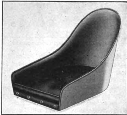
One of the Belfast racing seats designed for cars remodeled into raceabout or speedster types. They are light but strong in construction and the cushion is removable
